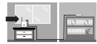
Attach the antennas to the two ports of the Cel-Fi unit and place one in the window and the other in the area where coverage is required.
